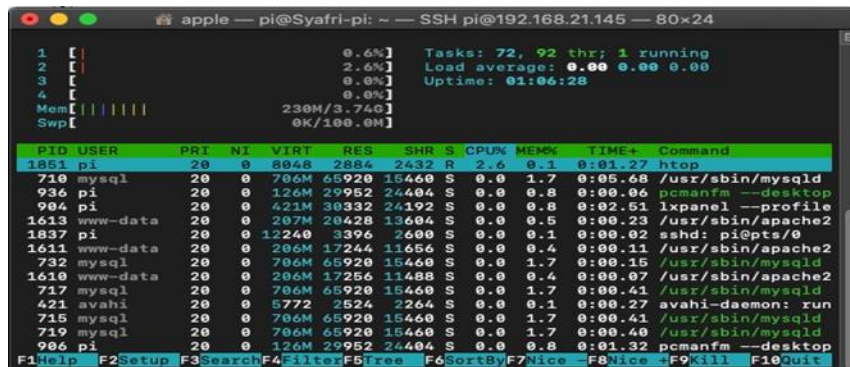
Gambar 13. Pengujian Beban Server Diakses Multi User
